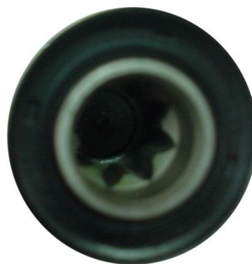
Steering pump with good splines
