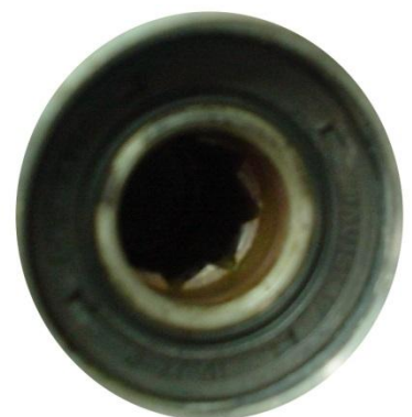
Steering pump with damaged splines
